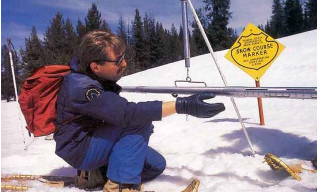
The snow-water equivalent is measured at a site in January. Photo/Natural Resources Conservation Service
